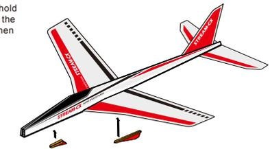
Attach the hook for the elastic, and the fin to hold the plane by, to the specified positions.
