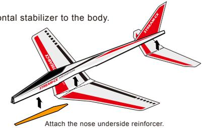
Attach the nose underside reinforcer.
